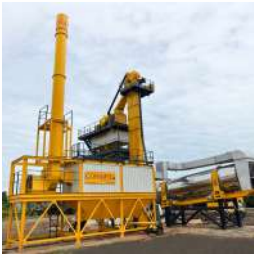
Asphalt Batch Mix Plant
